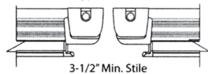
Double Door with Two Vertical Rod Type Exit Devices
